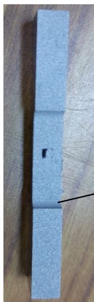
Figure 24. UTS test coupon
