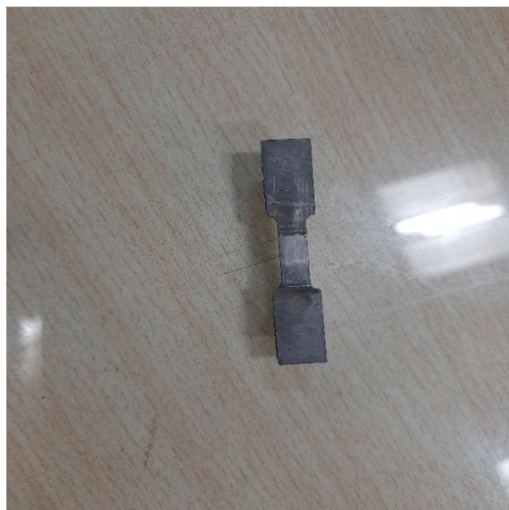
Figure 39. UTS test coupon of confirmatory test
