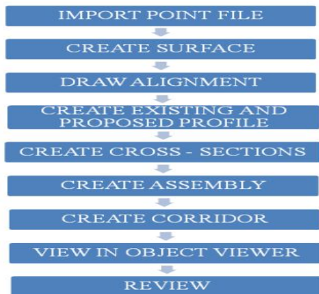
Figure-03 Flow chart of Geometric design in Civil 3D Software
