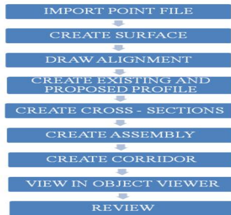
Figure-03 Flow chart of Geometric design in Civil 3D Software
