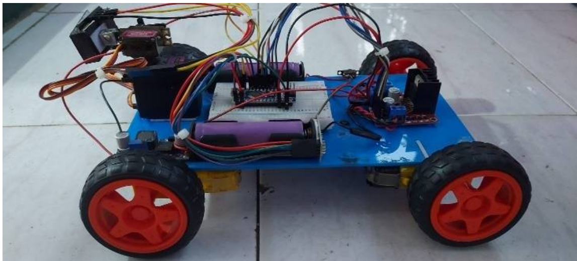
Fig. 11. Gesture-based Surveillance Car with ESP32 Camera module
