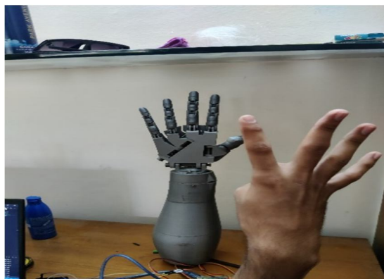
Fig 12: - Shows Testing of hand (4 finger as input)
