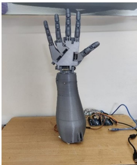
Fig 6: - gesture replicating robot arm
