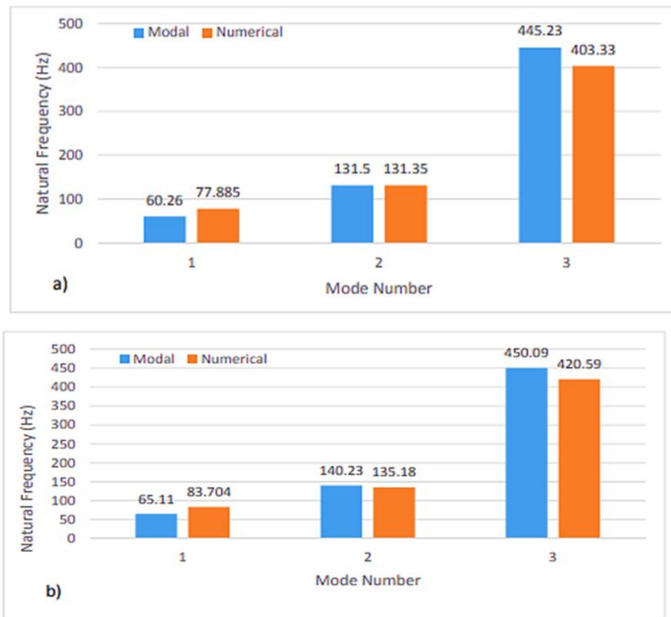
Fig. 10: Comparison of modal and numerical natural frequencies for a) GFRP and b) Hybrid GFRP composites
