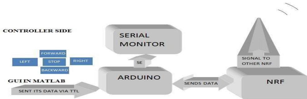
Fig. 3.1 Controller side block diagram
