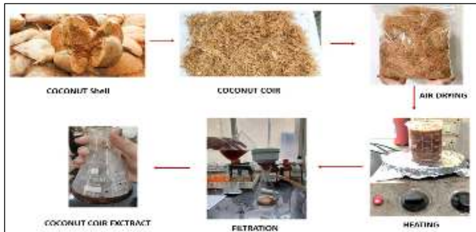
Fig-2 Coconut Coir Extract preparation
