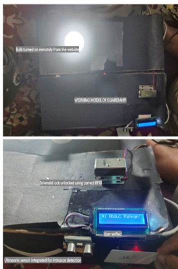
Fig. 12 Physical Model of the GuardianPi System
