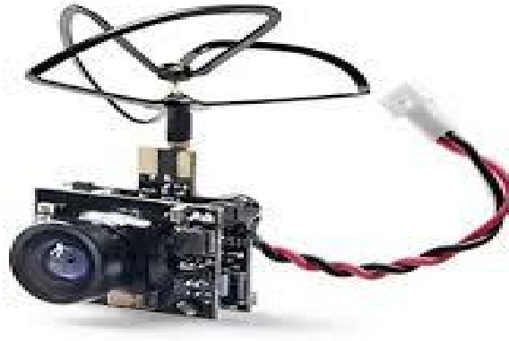
Fig. 4. FPV Camera with built-in transmitter.
