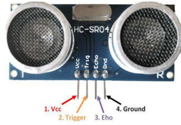
Figure 3: Pin layout of Ultrasonic sensor
