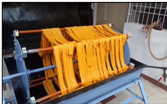
Figure 5: Coloring in Hank Dyeing Machine (Source: Author)
