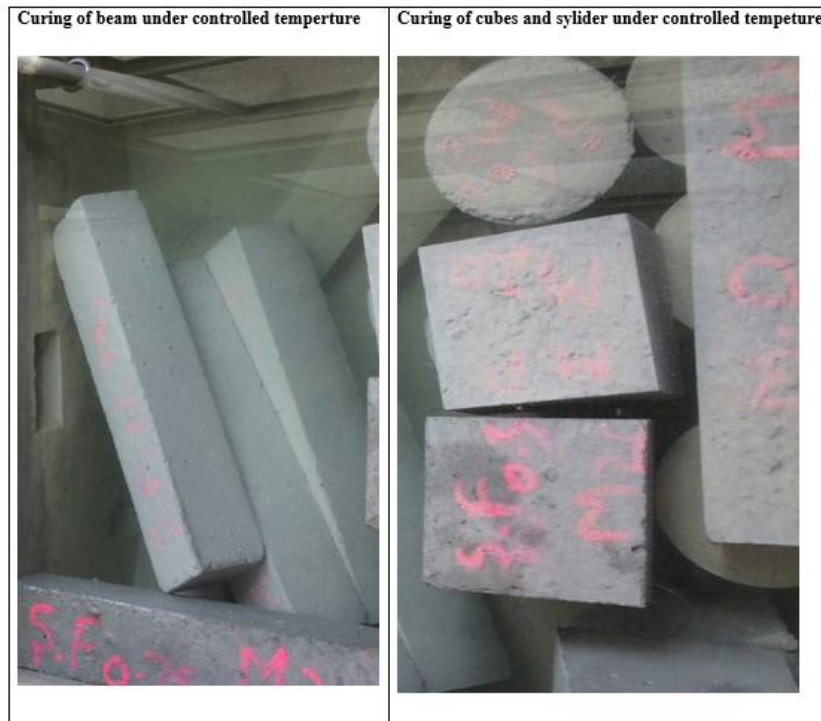
Fig.5 Specimen is placed in a curing tank.
