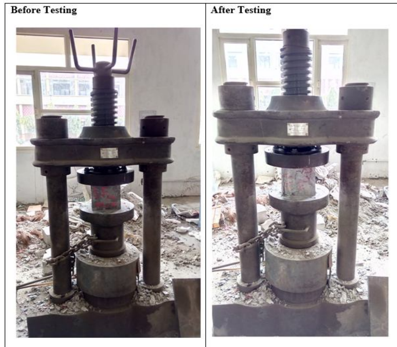
Fig.6 Compression Cube Test
