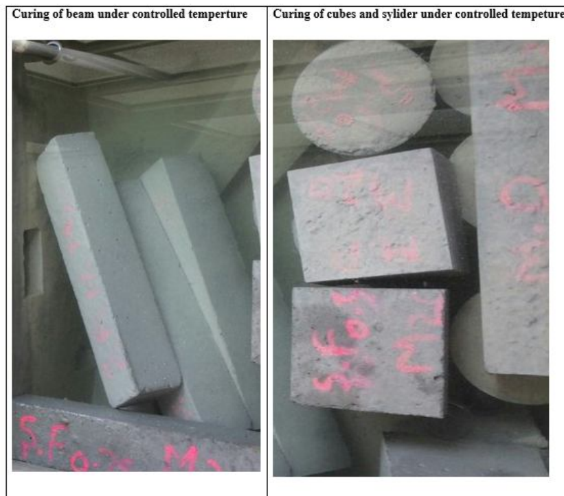
Fig.5 Specimen is placed in a curing tank.
