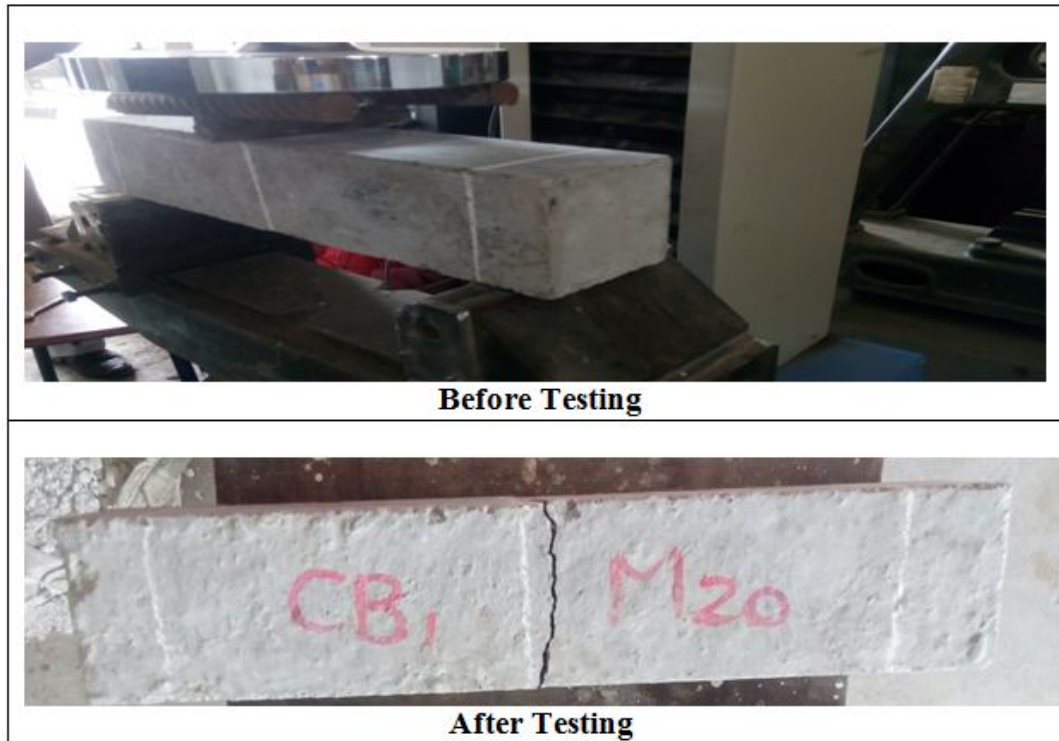
Fig. 10 Beam flexural test
