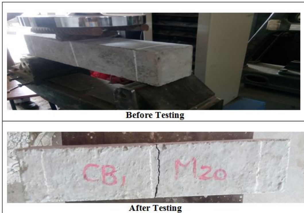
Fig. 10 Beam flexural test
