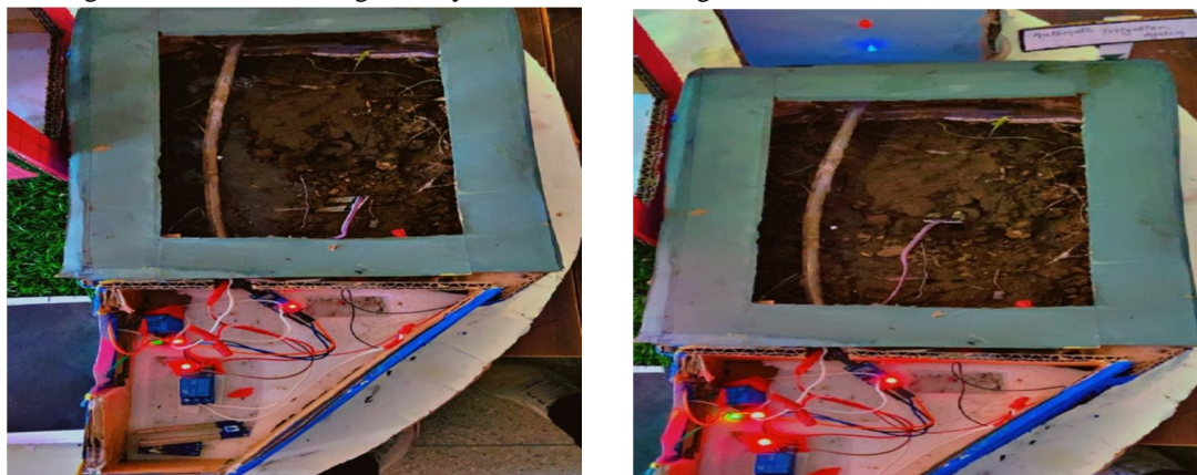
Fig.4 Automatic Irrigation System
