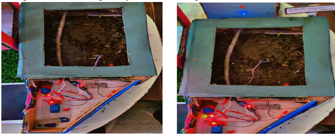
Fig.4 Automatic Irrigation System
