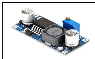
Fig. 11 LM2596S DC-DC Buck Converter Power Supply
