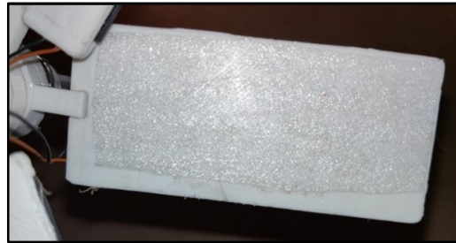
Fig. 15 Cleaning Material Sheet behind Solar Petal
