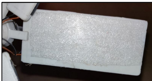
Fig. 15 Cleaning Material Sheet behind Solar Petal
