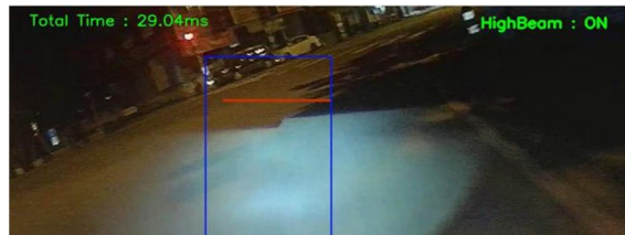
Fig. 4. Schematic diagram of driving far lights without vehicles ahead.
