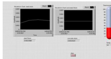
Fig 5.2 Strain corresponding to 500kg(5KN/M) while unloading
