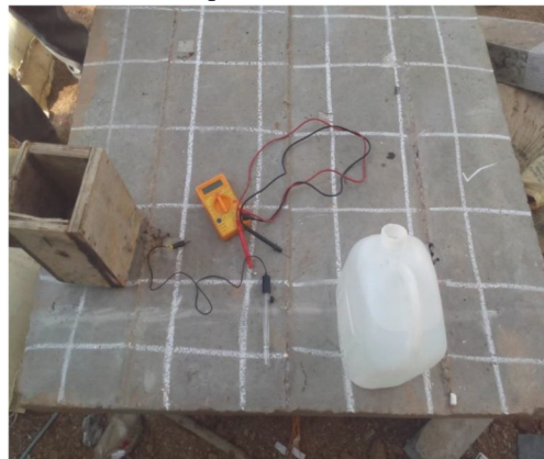
Fig 5.5 Prepared slab for measuring the potential difference at various locations of the slab using calomel reference electrode.
