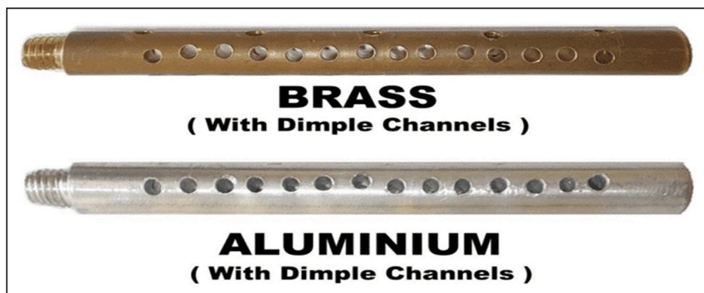
Fig.3. Pin fin with dimple channels
