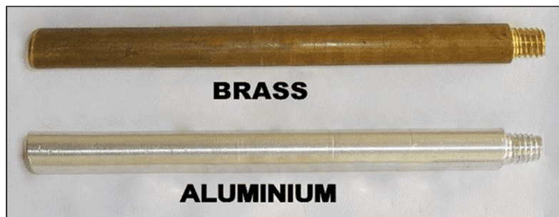
Fig.2. Pin fin without dimple channels
