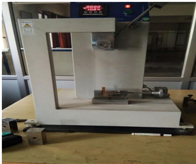
Fig. 2.1.2 Impact testing machine with Sample loaded condition
