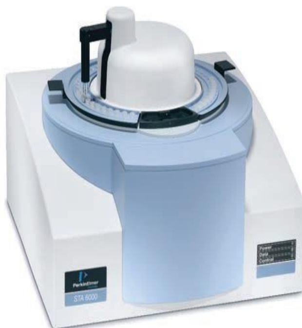
Fig. 2.2.2 STA 6000 used for DSC and TGA test
