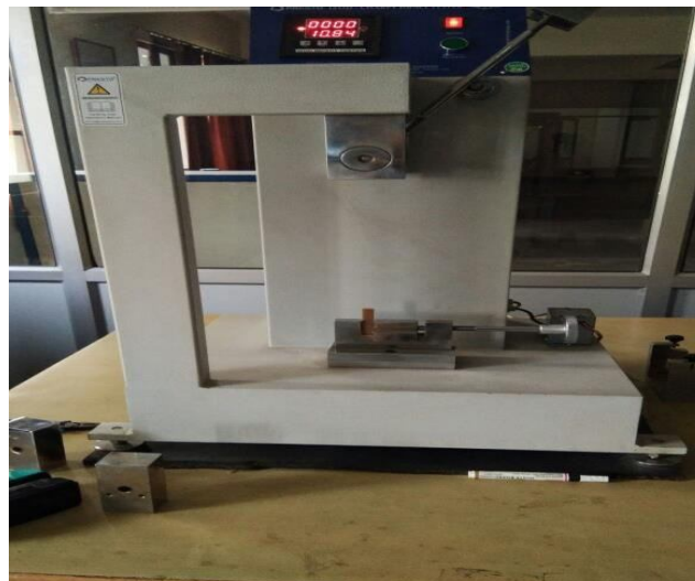
Fig. 2.1.2 Impact testing machine with Sample loaded condition
