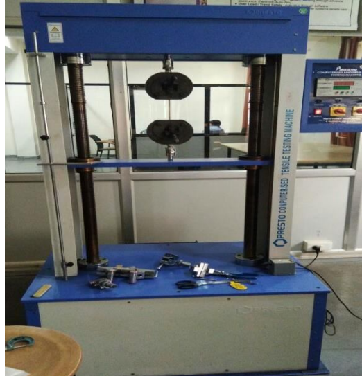
Figure 2.1.1 shows the UTM machine with the sample loaded for tensile testing.
