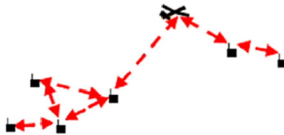
Fig. 1 Using UAV to relay between ground stations [1]
