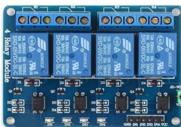
Fig. 3 Four channel relay module.
