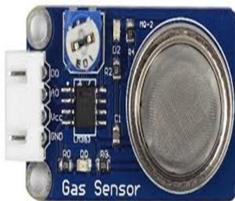
Figure 4: a MQ-2 sensor module
