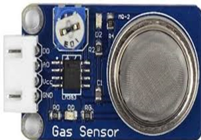
Figure 4: a MQ-2 sensor module
