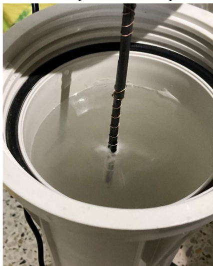
Fig.5.2: Oxygen generated at anode
