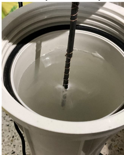
Fig.5.2: Oxygen generated at anode
