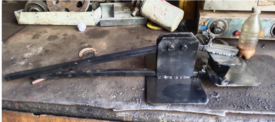
Fig 7. Developed Model of Hoof Cutter
