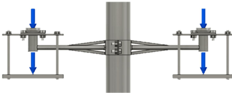
Fig 4: Load at the Turbine Location
