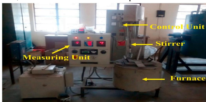
Fig. 2. Stir casting process setup.
