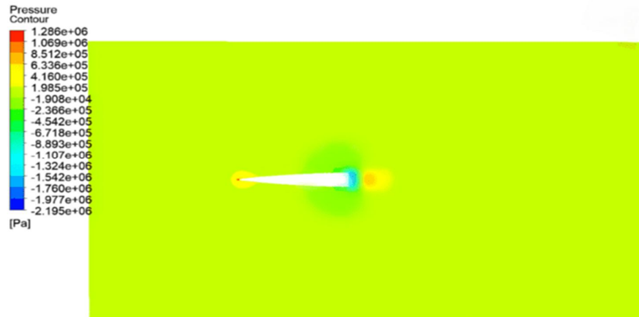
Figure 35. Pressure Contour of LD-Haack Series Nose Cone at Mach 9
