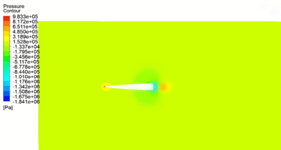
Figure 34. Pressure Contour of LD-Haack Series Nose Cone at Mach 8
