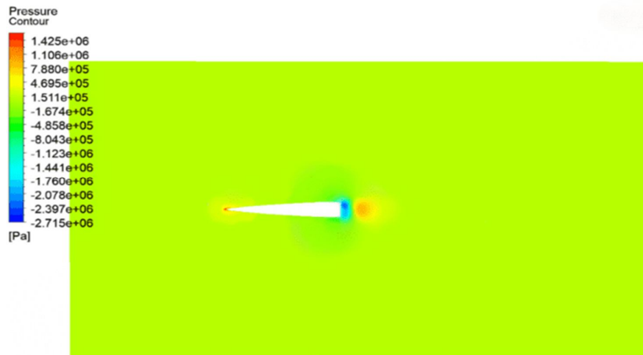
Figure 36. Pressure Contour of LD-Haack Series Nose Cone at Mach 10
