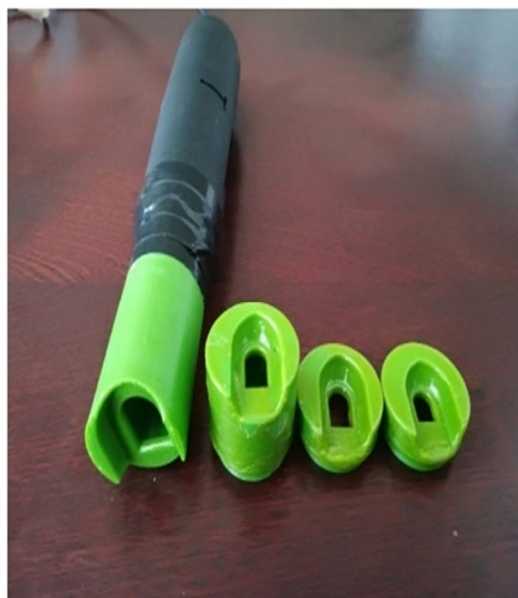
Fig 8. Baby fingerprint acquisition device without contact
