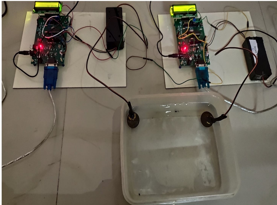
Fig 4.5 Water Data Communication Module
