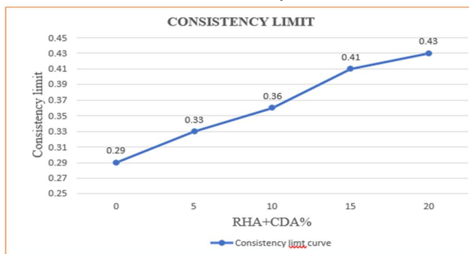
Fig. 3: Consistency curve for RHA+CDA concrete mix
