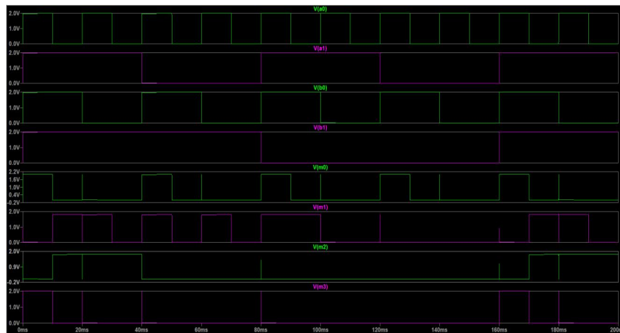
Fig. 6 Simulation results for the proposed Multiplier Circuit
