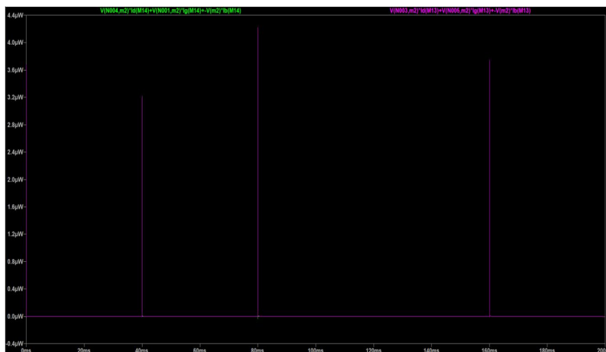
Fig. 13 Power dissipation at m2 for Multiplier Circuit
