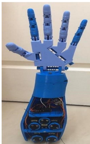
Figure 6: 3-D printed Prosthetic Hand
