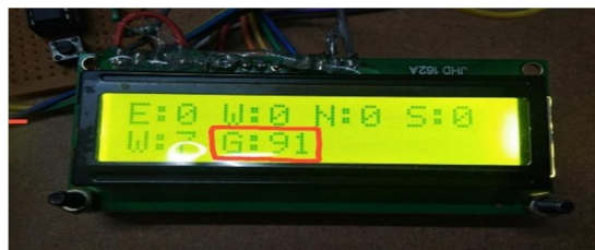
Fig. 9. LCD displays amount of air pollution
