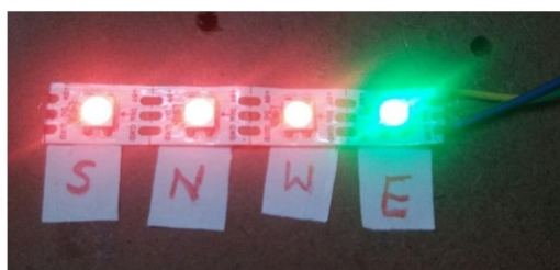
Fig. 11. LED displays green at east direction
