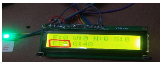
Fig. 10. LCD displays highest density direction
