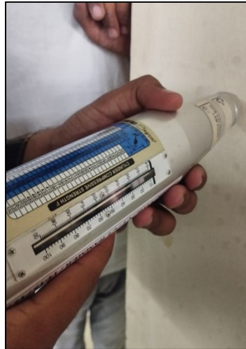
Fig. 4. Rebound Hammer Test
