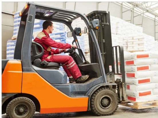
(b) Forklift truck operator without helmet
