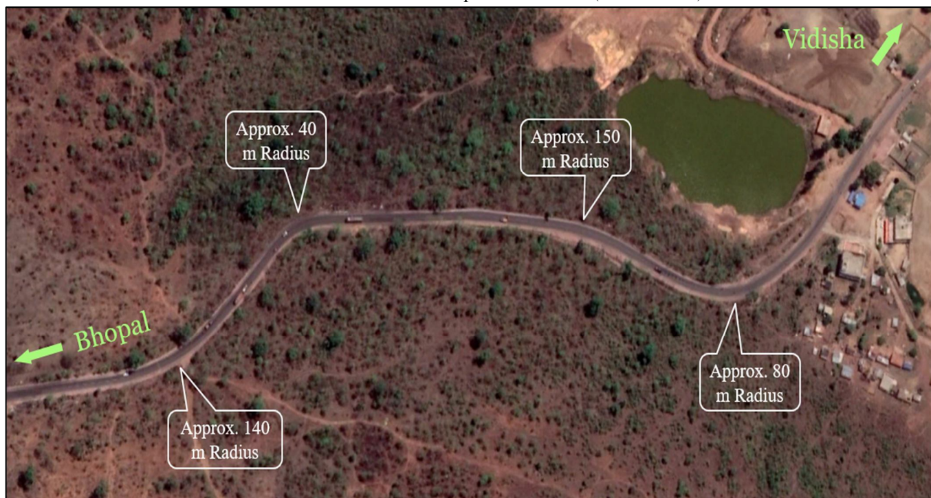
Figure 3: Horizontal curves deficiencies
