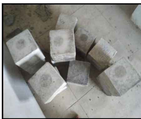
Figure 4.4: Cubes After Completion Of Curing Period
