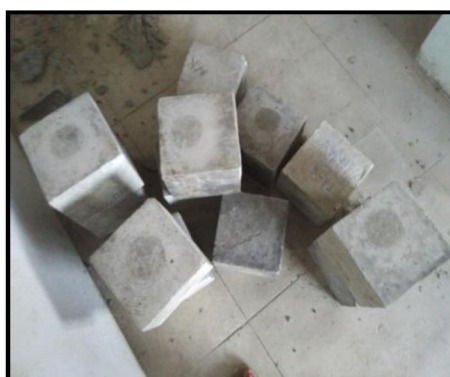
Figure 4.4: Cubes After Completion Of Curing Period
