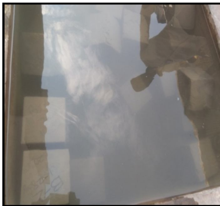
Figure 4.3 Curing Of Cube Specimen
