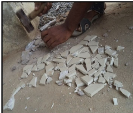
Figure 3.9: Manual Crushing Of Waste Tiles
