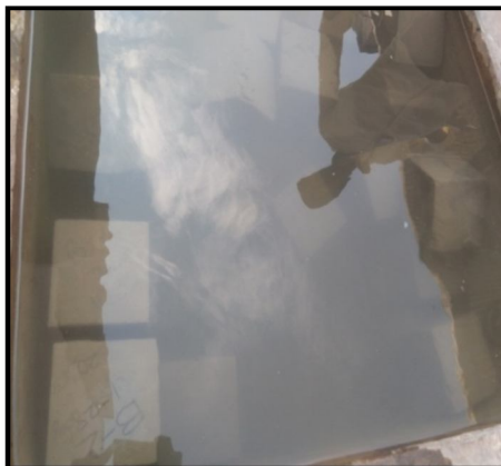
Figure 4.3 Curing Of Cube Specimen
