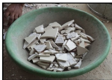
Figure 3.10: Materials Separated After Crushing
