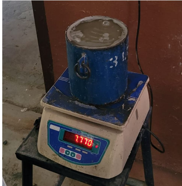
Fig 7: Specific gravity test for Fine aggregate
