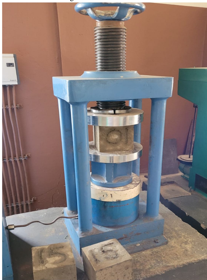
Fig 12: Compressive strength test on CTM
