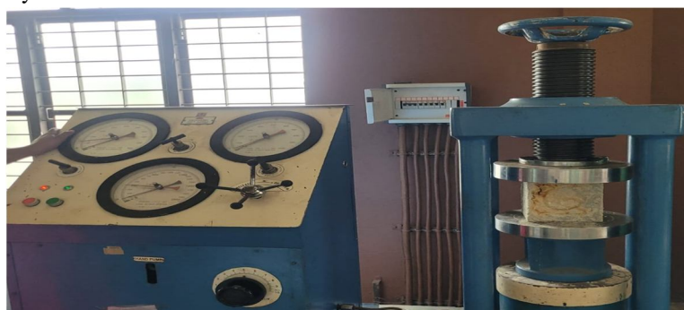
Fig 17: Testing the compressive strength of specimens subjected to durability test
