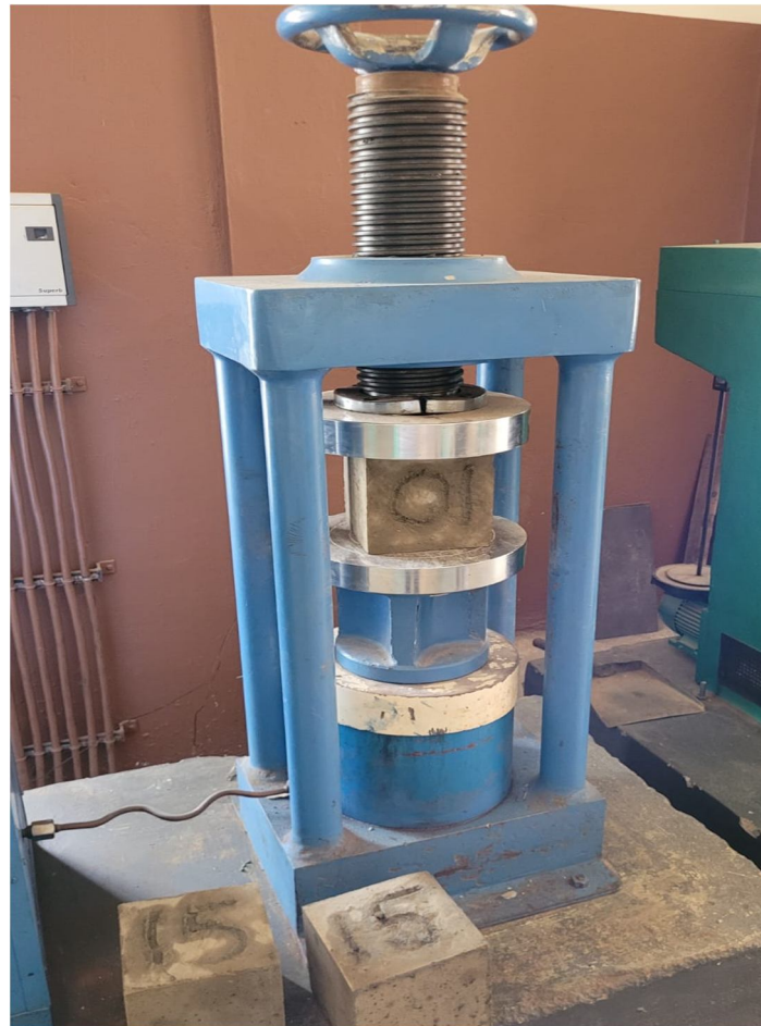
Fig 12: Compressive strength test on CTM
