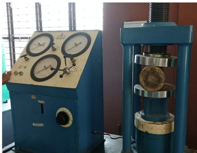
Fig 15: Split tensile strength test on CTM
