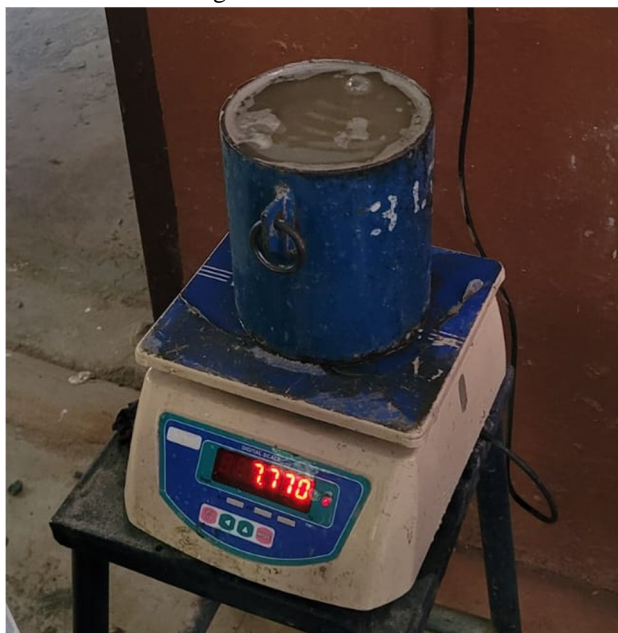
Fig 7: Specific gravity test for Fine aggregate
