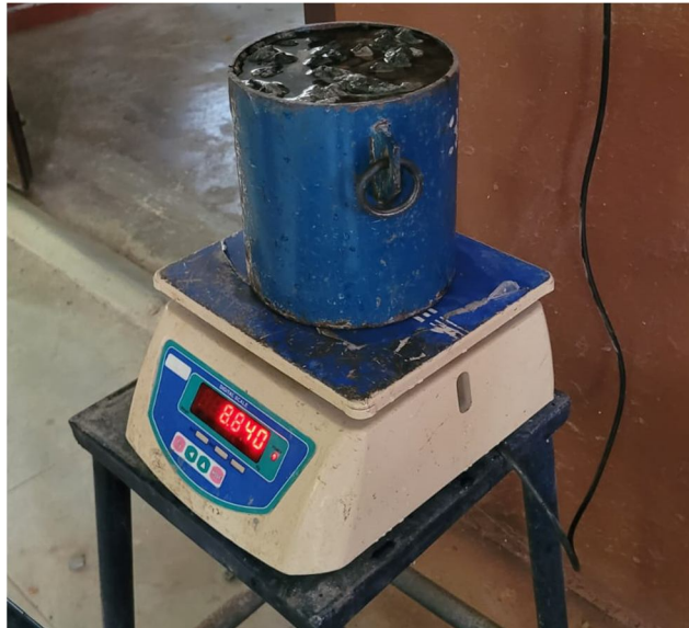
Fig 8: Specific gravity test for Coarse aggregate
