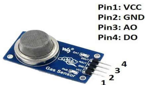
fig.4 Pin diagram of MQ2
