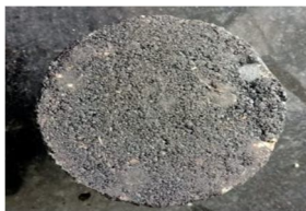
Fig 17: Casted bituminous mould
