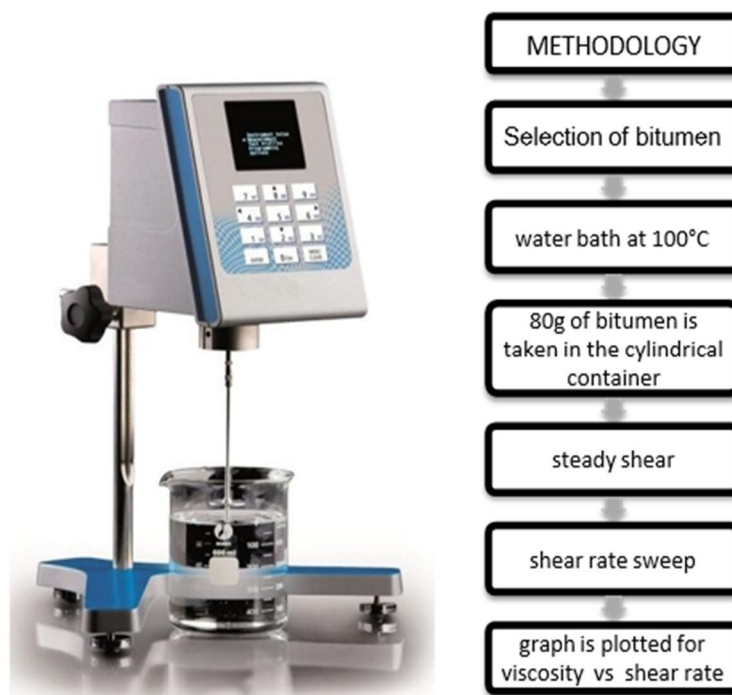
Fig 1: Viscometer and its methodology
