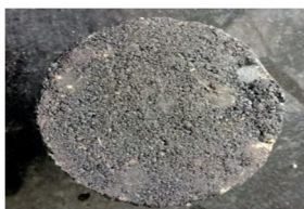
Fig 17: Casted bituminous mould
