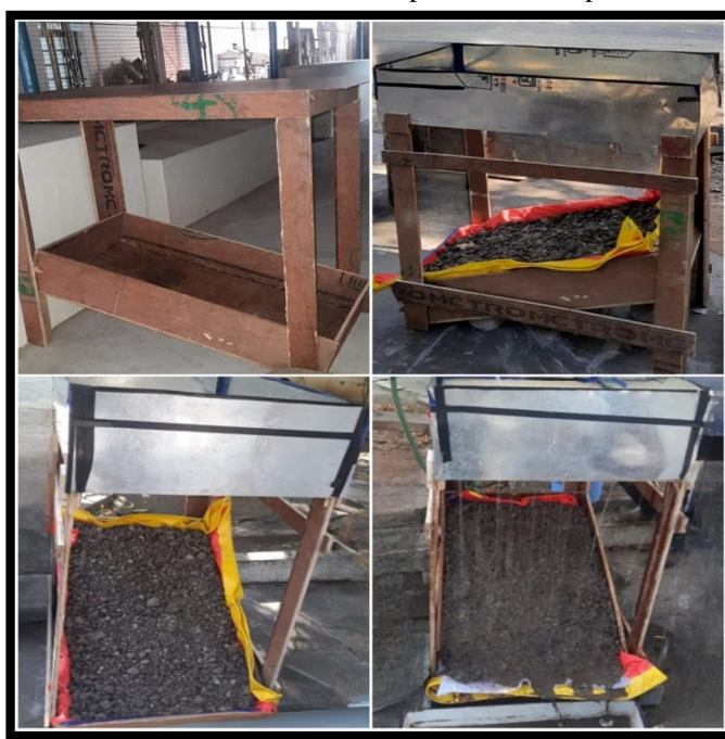
Figure 1: Experimental Setup and Artificial Rainfall in Slope Model
