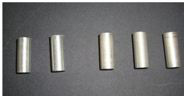
Figure 2.3: Wear Testing Pins
