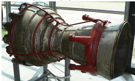
Figure 4.4: Convergent-divergent nozzle design: CD Nozzle
