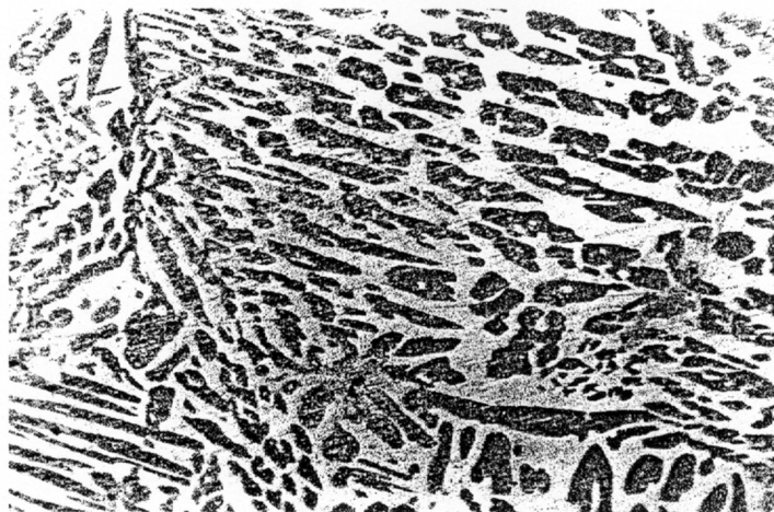
Fig 5 A few pits observed in as cast sample dipped in 3.5% NaCl + 5 % H 2 SO 4 for 10 hours ( Mag 100 X )
