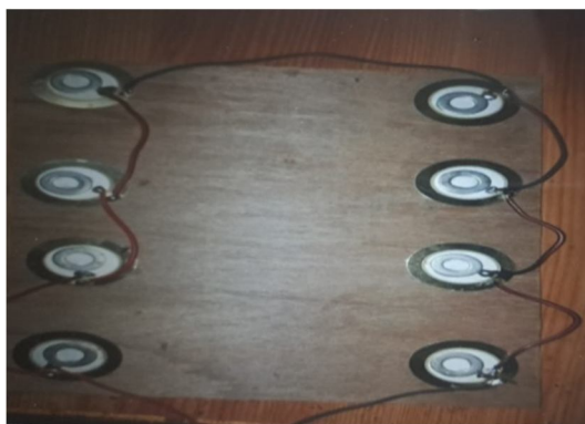
Fig: piezo sensor connections
