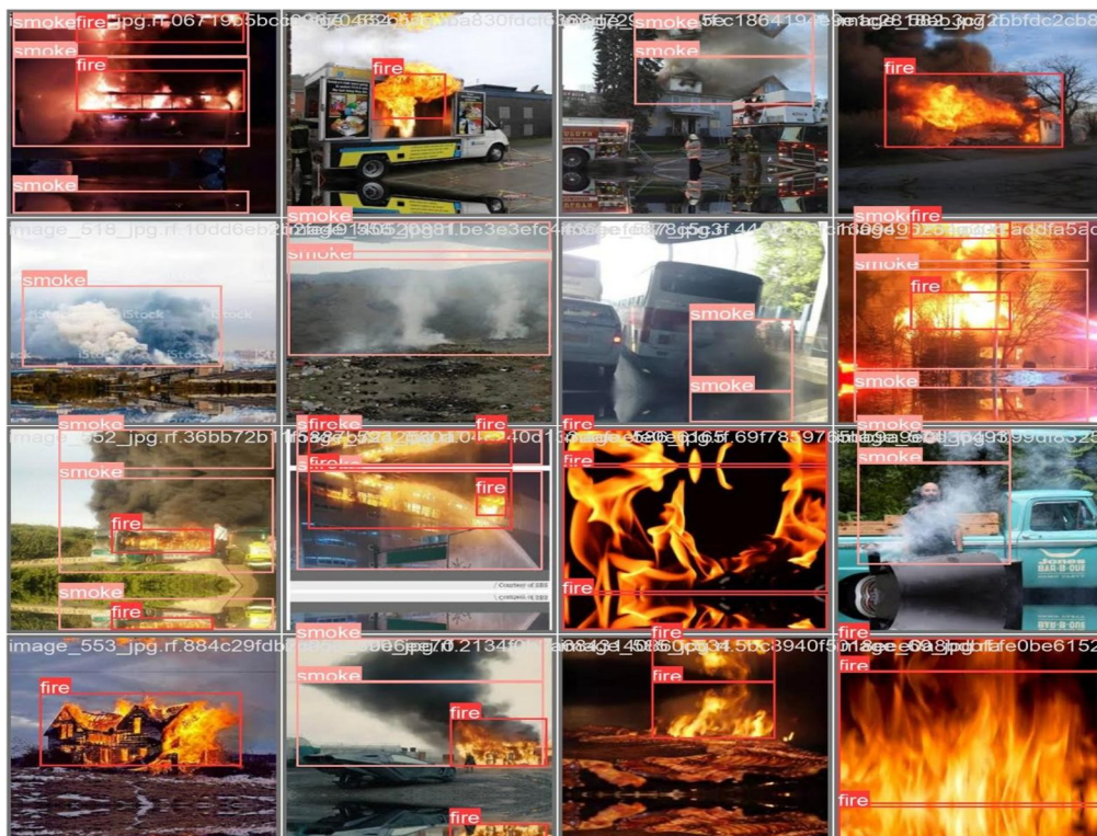
Fig 8:- The result of proposed model for fire and smoke detection
