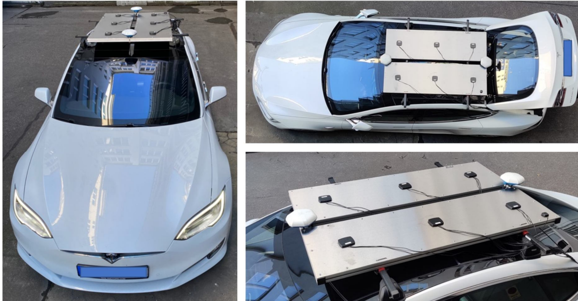
Figure 1. The antenna setup of the vehicle.
