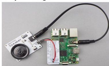
Fig 4. Speaker for Raspberry Pi
