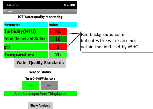
Fig. 3 Mobile app displaying water quality parameters on a real time basis
