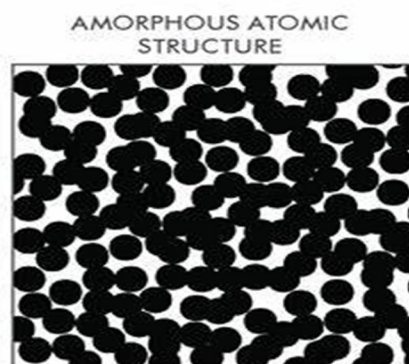
Atomic structure of glass materials.
